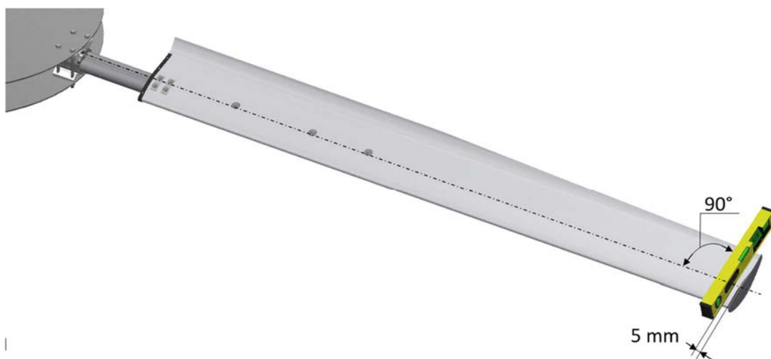
Figure 2.19: positioning of protractor on blade
