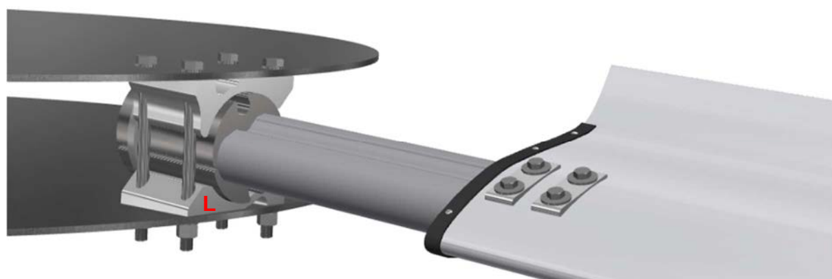
Figure 2.18b: blade installation on hub: mounted
