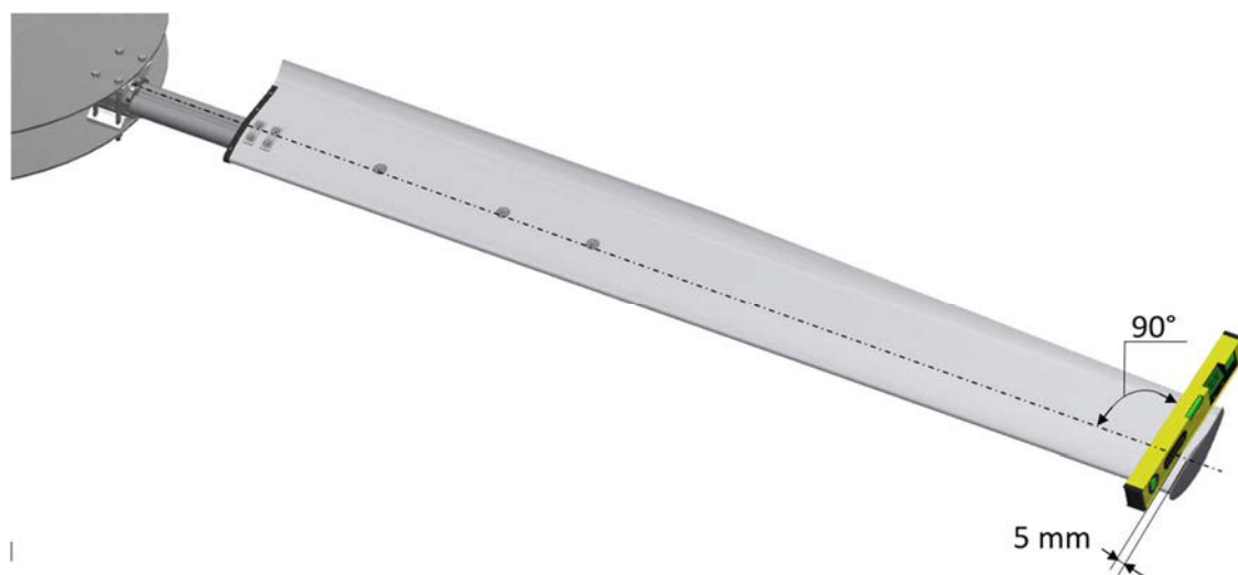
Figure 2.19: positioning of protractor on blade
